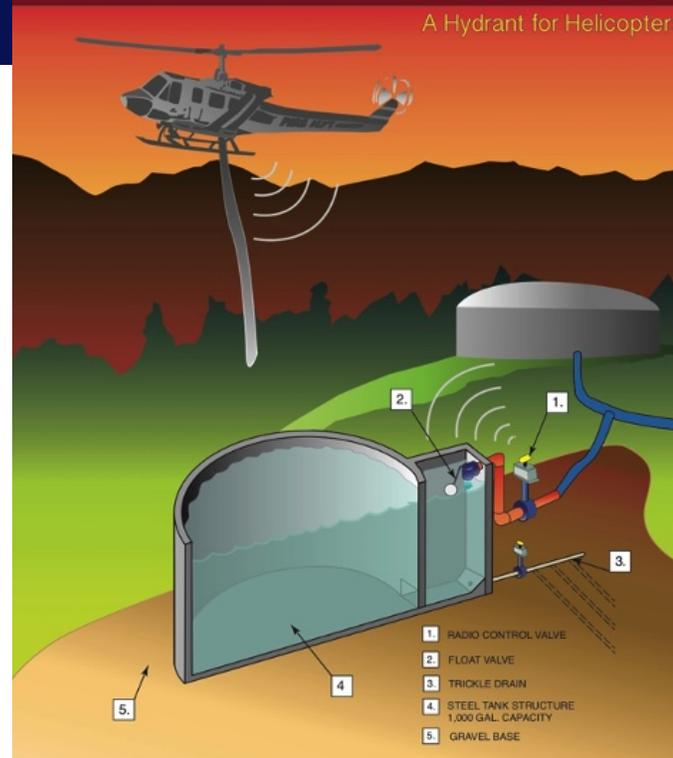
To meet this critical need to get water onto a fire fast, we are building a Heli-Hydrant. This is an above ground tank with specialized valves and piping that allows a firefighting helicopter to fill up with water for fire suppression. Having this type of local resource will reduce flight times between trips. A lot of fires seem to start along the I-15 corridor so this facility will be in an ideal location above Pala Mesa.
