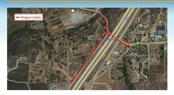
Scope of Work: Replace 3,788 feet of 30-inch and 27-inch pipelines that are severely corroded using CIPP technologies. In addition, the project would add three (3) new isolation valves.
